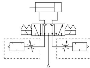
Residual pressure behind the exhaust needle may cause check valve malfunction in the "Perfect Valve".
