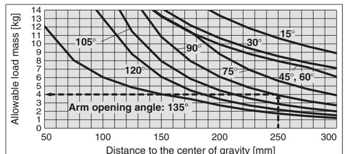
**Calculation example** Bore size: 63, Arm opening angle: 90°, Distance to the centre of gravity L: 250 mm
