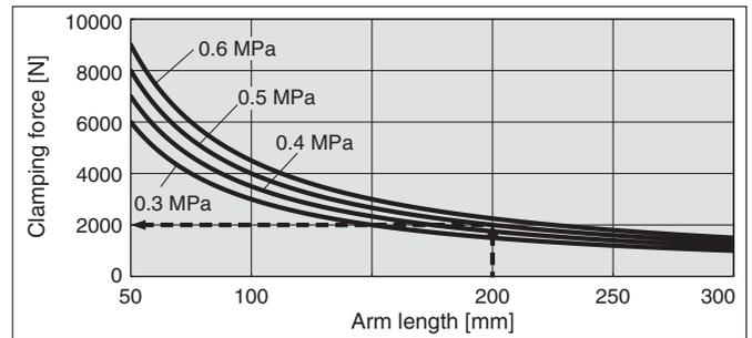
**Calculation example** Bore size: 63, Arm length: 200 mm, Operating pressure: 0.5 MPa
