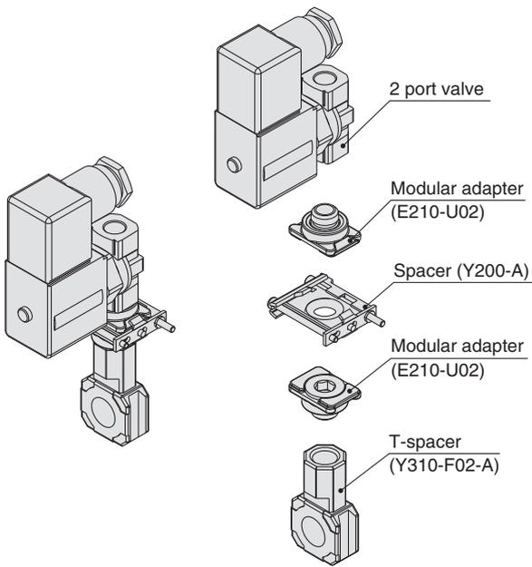
**Ex. 6 T-spacer to downward face mounting (2)**
