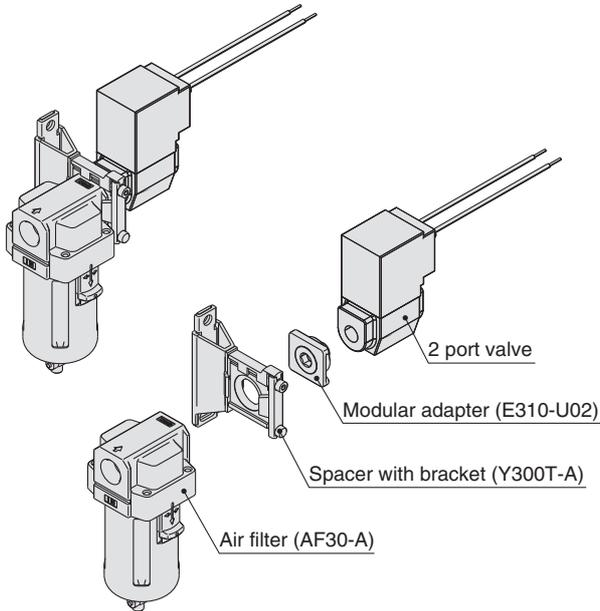
**Ex. 2 2 port valve connection to air tank**
