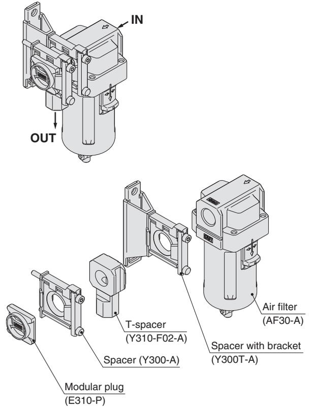
**Ex. 7 Downward face mounting for L-shaped piping adapter**
