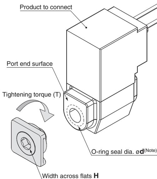
Note) The surface roughness of the seal surface of the product to be mated to the modular adapter must be less than Rz25.
