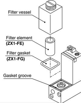
Filter assembly (Filter vessel + Filter element)
