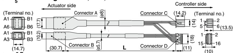
**LE-CP-<sup>8 B</sup>/<sub>A C</sub>**/Cable length: 8 m, 10 m, 15 m, 20 m
