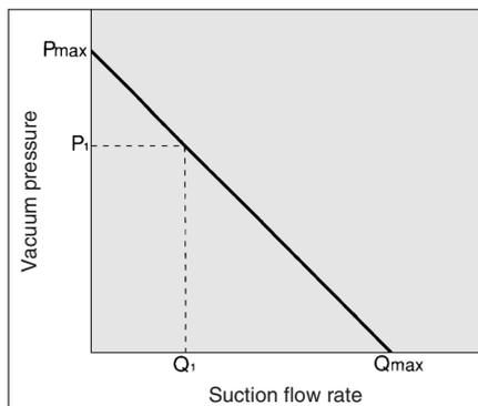
Flow rate characteristics are expressed in ejector vacuum pressure and suction flow. If suction flow changes, the vacuum pressure will also be changed. Normally this relationship is expressed in ejector standard operating pressure use. In the graph,  $P_{max}$  is maximum vacuum pressure and  $Q_{max}$  is maximum suction flow. The values are specified according to catalogue use. Changes in vacuum pressure are expressed in the below order.
