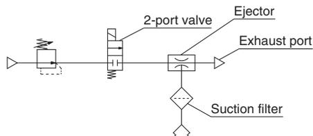
2-port valve is used to generate and stop the vacuum. Vacuum is released to the atmosphere. A suction filter is installed to protect the ejector.
