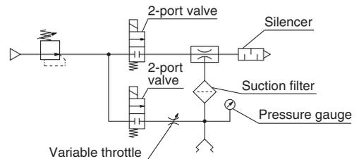
Vacuum generation and vacuum release are controlled by a supply valve and release valve. A pressure gauge is installed to visually check the vacuum pressure during adsorption. The suction filter should be mounted to the location where the collected dust should not flow back due to the release of air. (When using the 3-port valve, seal the R-port of the release valve.)
