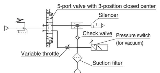
5-port valve with 3-position closed centre is used to control the vacuum generation and release. A check valve is installed to the vacuum port to prevent vacuum pressure from being reduced when the supply valve is OFF\*1. A pressure switch is installed in the vacuum circuit to detect pressure. A suction filter should be mounted to the position where the duct collected by release air can be flushed by released air.
