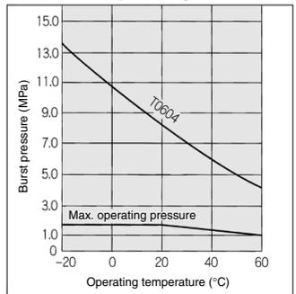
\* Maximum operating pressure is 1/3 max. of burst pressure at 60°C, considering the safety ratio.
