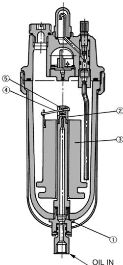
The oil that has been pumped from the tank passes through felt (1) where it is filtered, and is fed into the case through nozzle (2). When the volume of oil reaches a certain level, float (3) ascends, valve (5) descends via lever (4), nozzle (2) closes, and the feeding of oil stops, thus completing the oil feeding process. When the oil inside the case is consumed, float (3) descends, valve (5) ascends via lever (4), allowing oil to be fed from nozzle (2).
